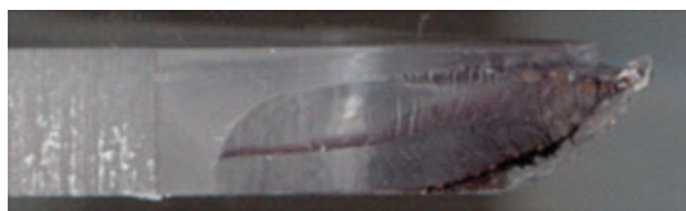
Figure 9 Radial crack surface area for energy estimates. Sample thickness = 5.75 mm. [Color figure can be viewed in the online issue, which is available at www.interscience.wiley.com .]
